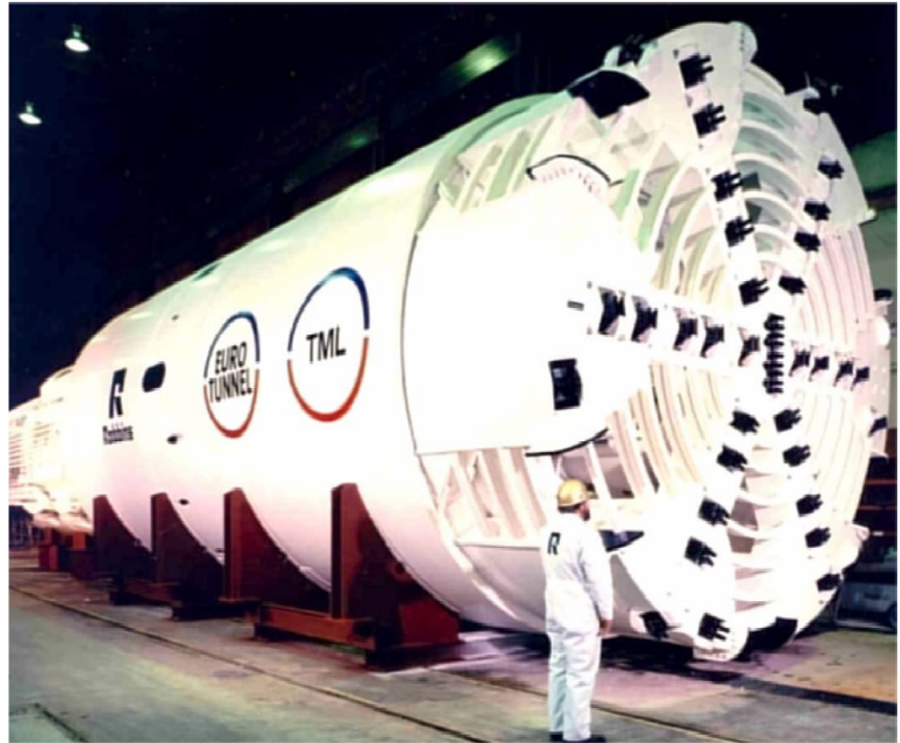
Figure 92. Robbins/Komatsu Channel Service Tunnel Shield, France. (Courtesy The Robbins Company)
